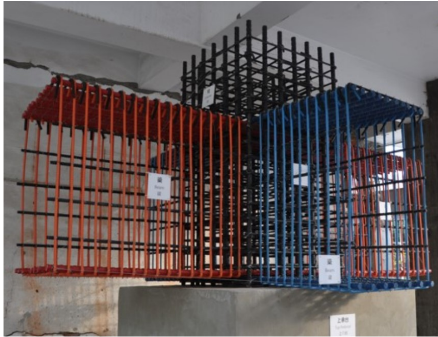
Figure 1. Increase in the cross-sectional area and number of reinforcement girders, columns, and girder-column joints due to the increase in ground vibration fortification levels (Hsu, et al., 2023).
